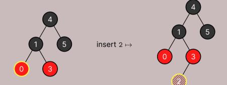
Well, if we want to rebalance this tree in the same way, we have to move the 2 up to 1's current position. But what should we do with the 0 node?
